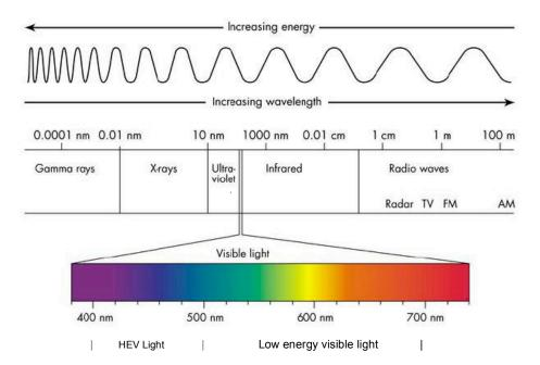
The human eye responds to only a small portion of the entire electromagnetic energy spectrum the portion described as the visible light spectrum.
