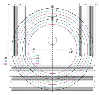
**Centering:** Center the Sync lens according to the monocular distance PD and make sure that the marking line overlaps the center of the pupil when looking straight in horizontal (zero) distance direction.
