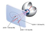
Digital Ray Path performance This last drawing shows the effect of a lens with the same prescription, calculated with Digital Ray-Path, ground with Free-form equipment. The Power experienced by the wearer is stable on the whole lens, providing perfect vision for every direction of sight.
